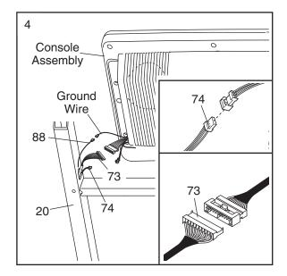
Set the console assembly on the Uprights (20). Make sure that no wires are pinched. Finger tighten a Console Bolt (72) with a Star Washer (67) into the lower hole in each Upright (only one side is shown).
